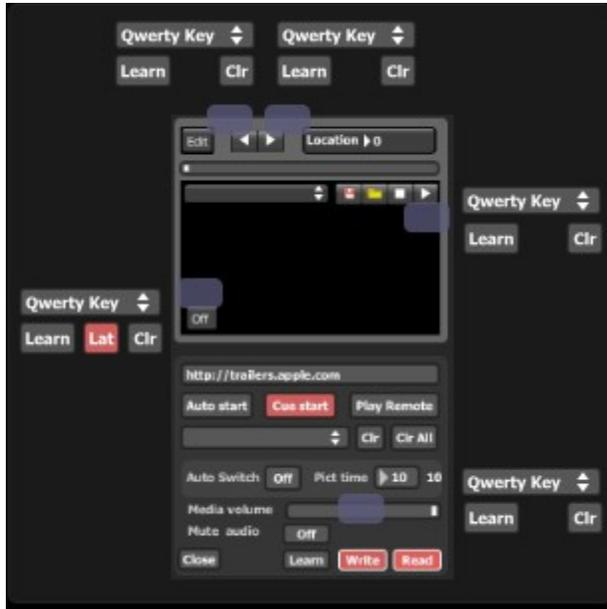
On the learn panel you will see small blue boxes showing the PixelNet control that can be controlled by an external source.
