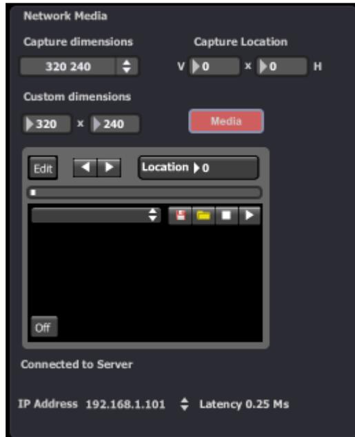
When Pixelwarp and Pixelnet are running PixelNet's panel will display "connected to server". If no IP address is displayed, click the word IP Address. The addresses of servers that are connected will fill the pull-down menu. Select the IP of the server you wish to send media to. To the right is the delay or latency you will experience with current settings and media
